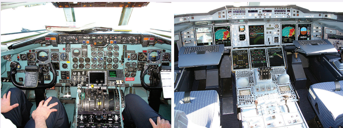
FIGURE 14.4. Airplane cockpits. Initial design of the airplane cockpit (left); the digital design of the airplane cockpit (right), which has taken human factors into account. [“cockpit” by University of Saskatchewan is licensed under CC BY-NC-SA 4.0. ]
