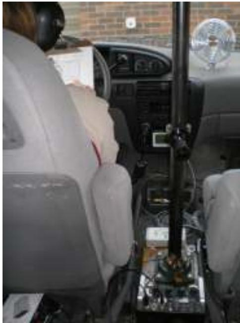
Figure 1b – Inside of telemetry vehicle with receiver, null/peak antenna box (white) and compass display (under radio)
