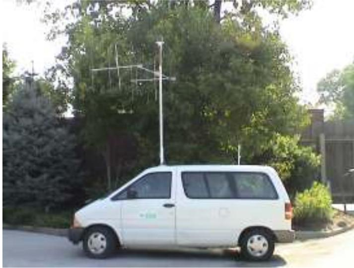
Figure 1a – Telemetry Vehicle with null/peak antenna system and electronic boat compass on the top of the mast.
