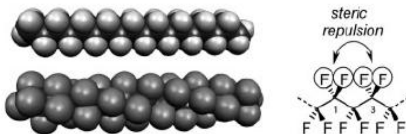
Fig. 2. The zigzag confirmation of octadecane (above) compared with the helical perfluorooctadecane (below). [1-1]
