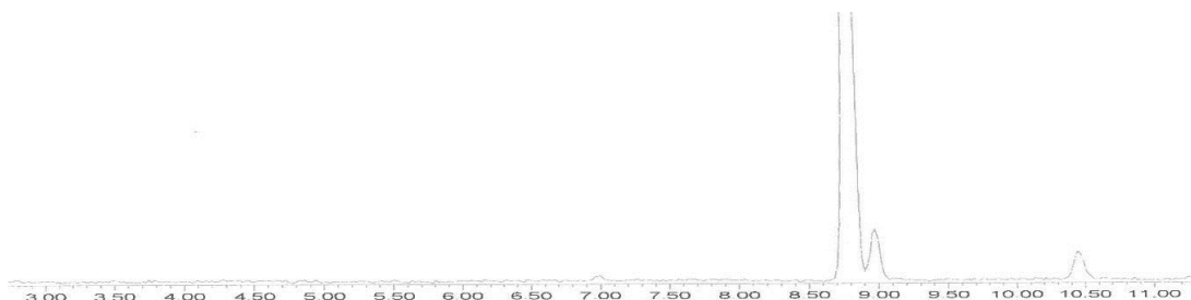
Figure G-1. GCMS trace of the LBAM pheromone using total ion current at T/K = 483 , solvent not shown.
