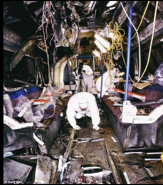
Evidence of bomb explosion from under train.
