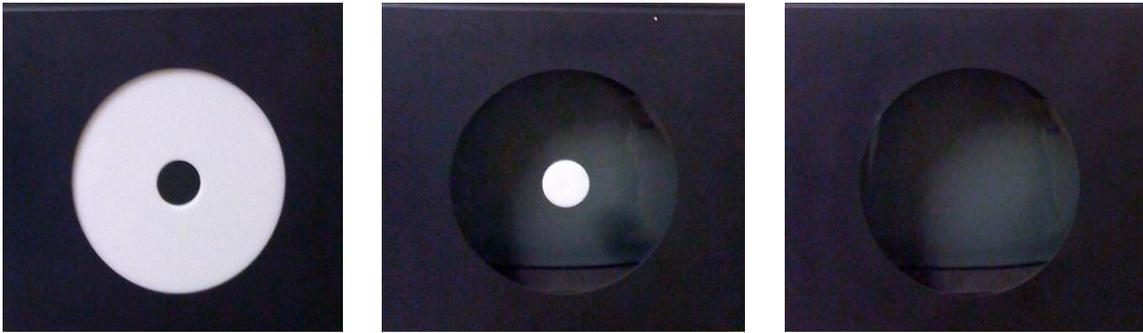
**Figure 4** shows the apparatus that was attached to the front of the display screen for the two degree, ten degree, and full field targets.
