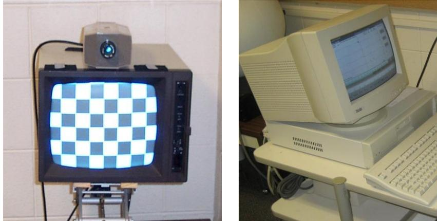
**Figure 2** shows a VEP apparatus. The monitor with the checkerboard pattern is what the subject views and the monitor with the waveforms is what the tester views.
