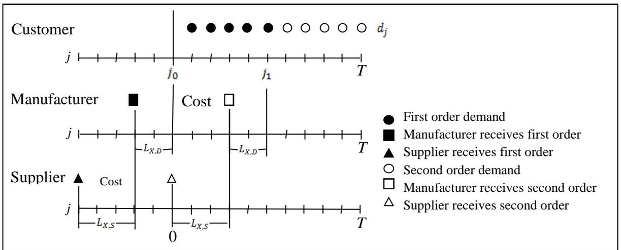
Figure 3.2: Timing of manufacturer and supplier costs relative to order delivery time
