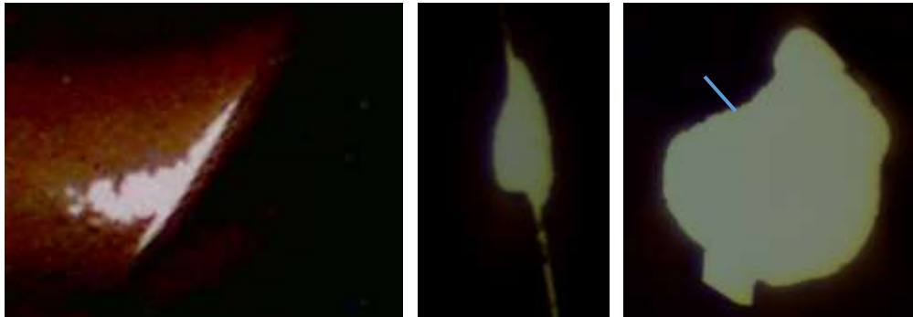
Figure 3.3: Amscope microscope pictures of perforation of specimens 1-3 (from left to right) for RGB analysis. Perforations on 200-500 micron scale. Blue line marks an example of line length, or “run”, as described below.
