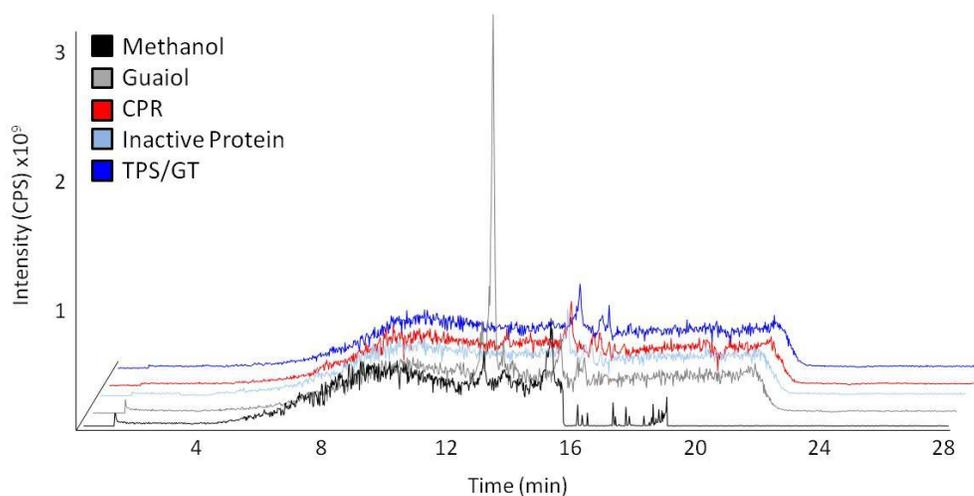
**Figure S4.6: LC-MS analysis of *Sf9* cell enzyme assay products. EPI scan at mass 415 Da.** Protein collected from *Sf9* cells were combined in an in vitro enzyme assay. The activity of the terpene synthase (TPS) and galacturonosyltransferase (GT) on FPP was compared to the activity the control cytochrome P450 reductase (CPR) and inactivated protein. CPS = counts per second.
