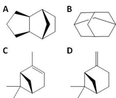
**Figure 6: Structural comparison of JP-10 fuel components and pinene isomers.** JP-10 aviation fuel consists of strained ring structures such as A) exo-tetrahydrodicyclopentadiene and B) adamantane. The monoterpenes C)  $\alpha$ -pinene and D)  $\beta$ -pinene have comparable structures and energy content. Figure adapted from Gao et al., 2015 (permission number 4340941292149) and NCBI Resource Coordinators, 2017.
