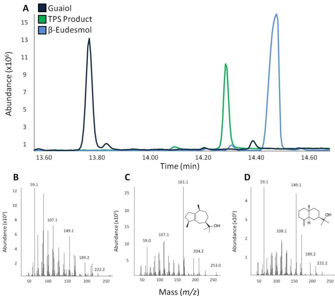
**Figure 13: Comparison of unknown terpene synthase product (TPS) to standards by GC-MS.** The retention time (A) and mass spectra of the unknown terpene synthase product (B) were compared to the standards guaiol (C) and  $\beta$ -eudesmol (D) by GC-MS analysis. Standards were purchased from Sigma-Aldrich. Mass spectra after background subtraction are shown.
