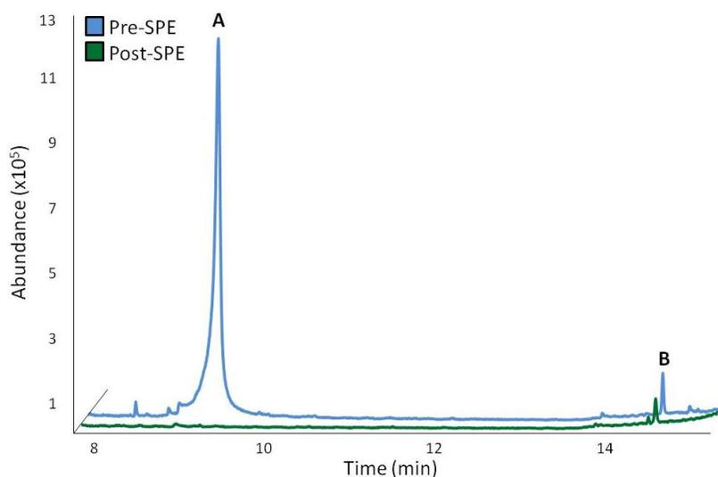
**Figure 16: GC-MS analysis of purification of cell extracts by reversed-phase solid phase extraction.** Contaminants such as indole (A) were removed from cell culture by SPE, isolating the terpene synthase product (B).
