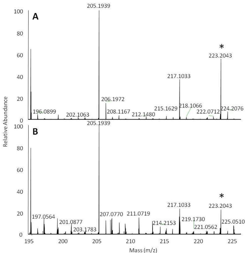
**Figure 17: Mass spectra of guaiol and the terpene synthase product during Q Exactive direct infusion. Guaiol (A) and the terpene synthase product (B) were analyzed by direct infusion MS using a Q Exactive. A precursor ion peak at 223.2043 Da (\*) is apparent when no collision energy is applied.**
