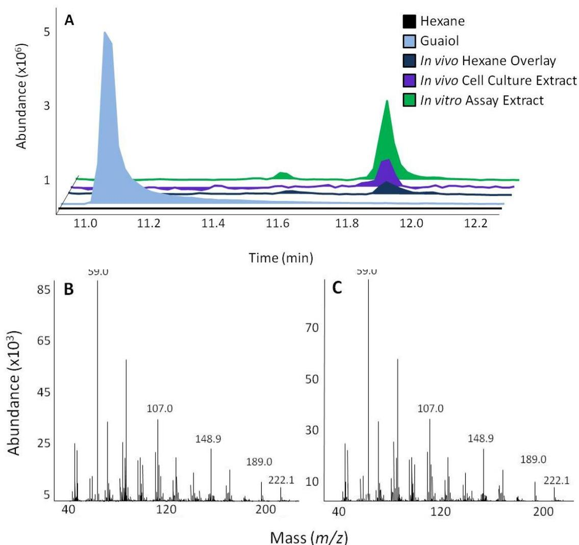
**Figure 14: Comparison of *in vivo* and *in vitro* enzyme assay products by GC-MS.** *In vitro* and *in vivo* enzyme assays were extracted using hexanes. (A) Comparison of the retention time of *in vivo* and *in vitro* enzyme assay products. (B, C) The mass spectra of *in vivo* (B) and *in vitro* (C) enzyme assay products were compared. Mass spectra after background subtraction are shown.
