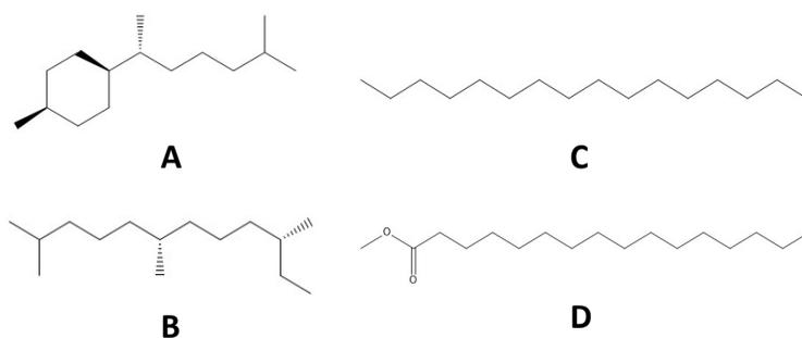
**Figure 5: Comparison of fuel structures.** The chemical structure of the terpenes A) bisabolane and B) farnesane are similar to the diesel fuel component C) hexadecane and D) methyl palmitate, a component of plant-based oils. Figure adapted from Peralta-Yahya et al., 2011 and NCBI Resource Coordinators, 2017.
