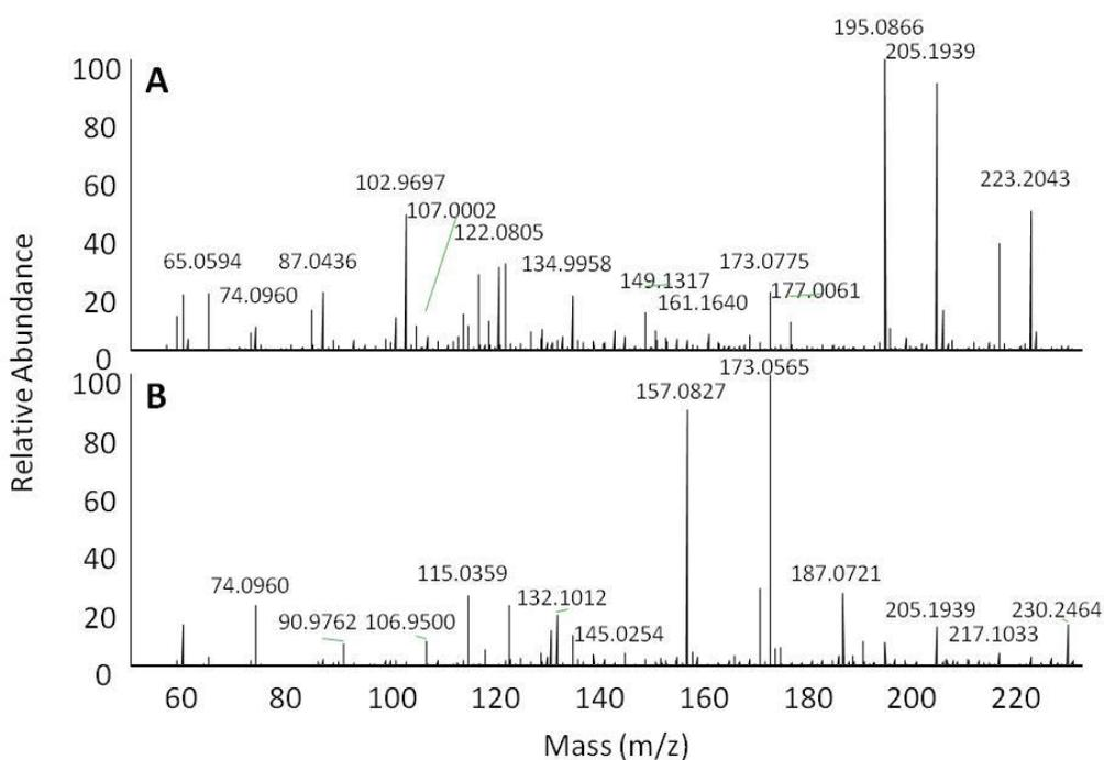
**Figure S3.5: Direct infusion MS analysis of the terpene product.** The standard guaiol (A) and the unknown terpene product (B) were analyzed by direct infusion into a Q Exactive MS/MS system. The resulting fragmentation patterns were compared in search of the unknown terpene product precursor ion.
