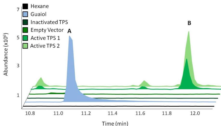
**Figure S3.4: GC-MS analysis of the products of FPP-supplemented enzyme assays.** The retention time of guaiol (A) and the product of enzyme assays with active terpene synthase (TPS) (B) were compared by GC-MS analysis.
