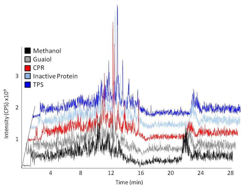
**Figure S4.3: LC-MS analysis of Sf9 cell enzyme assay products. EPI scan at mass 225 Da.** Protein collected from Sf9 cells were combined in an in vitro enzyme assay. The activity of the terpene synthase (TPS) on FPP was compared to the control cytochrome P450 reductase (CPR) and inactivated protein by targeted LC-MS analysis. CPS = counts per second.
