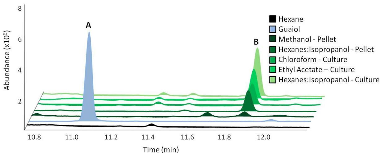
**Figure 15: Analysis by GC-MS of extraction method testing for maximum terpene yield.** Guaiol (A) was used as a standard to quantitate the concentration of the unknown terpene product (B) after extraction of cell cultures and pellets with chloroform, ethyl acetate, methanol, and hexanes:isopropanol.
