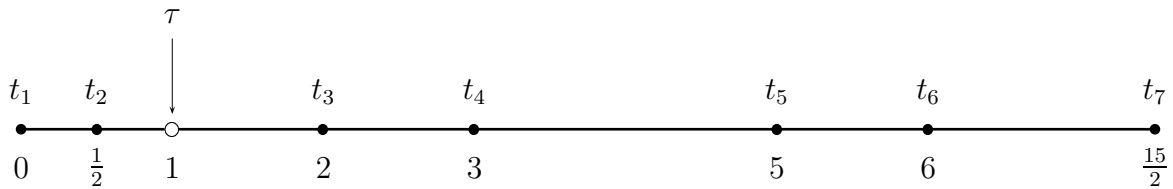
Figure 5.5: Knot sequence \{0, 0, 0, 0, \frac{1}{2}, 2, 3, 5, 6, \frac{15}{2}, \frac{15}{2}, \frac{15}{2}, \frac{15}{2}\} and new knot \tau = 1 .
