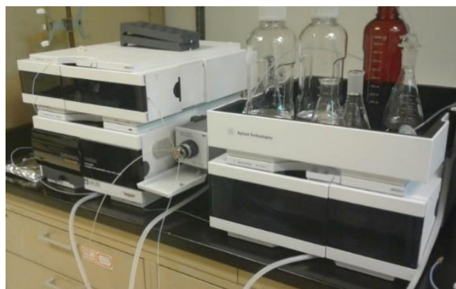
Scheme 1.44. The use of an autosampler as the mode for reagent delivery for the HPLC-based automation
